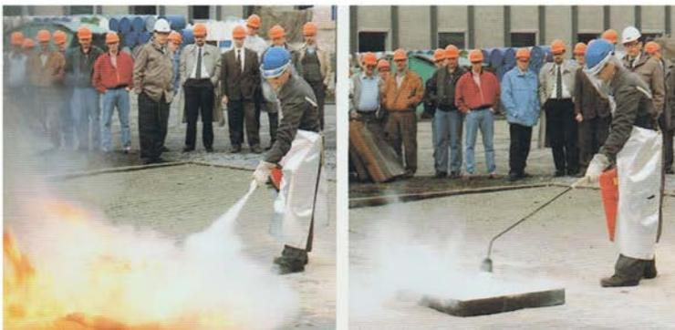
Compared with conventional powder extinguishers, this powder extinguisher with applicator reduces air turbulences over the source of the fire and in this way improves the extinguishing effect.
